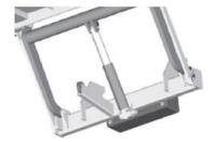
The one cylinder mid arm design provides great stability vs assembly weight ratio. The platform rotates on an adjustable roller for different bed heights.
